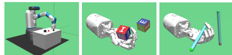
Figure 1: Examples of Goal-oriented RL tasks in OpenAI-Gym environment. The robot can be asked to move-fetch to a position, orient a block or play with a pen.
