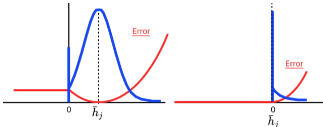
Figure 18: The variance of the noise and its contribution to the error. Graphical intuition behind Eqs. 23 & 25 .This term incentivizes neurons to be as negative as possible to avoid noise turning the neuron on.
