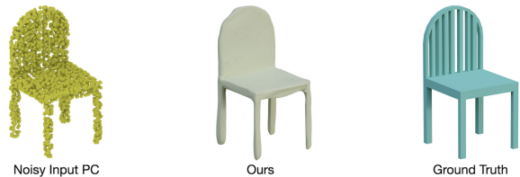
Figure 15. Failure case of NEURALSlice. As our method takes the discrete point cloud with noise as input, it is hard to discern the correct topology in such a challenging case.
