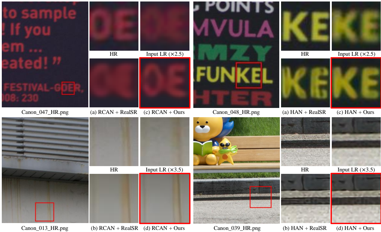
Figure 8. Qualitative comparisons on RealSR \times 2.5 and \times 3.5 test images that we acquired using the same data acquisition process for RealSR dataset (Cai et al., 2019). (a)-(b) SR results from RCAN and HAN trained with conventional dataset only. (c)-(d) SR results from RCAN and HAN trained with our synthetic dataset.
