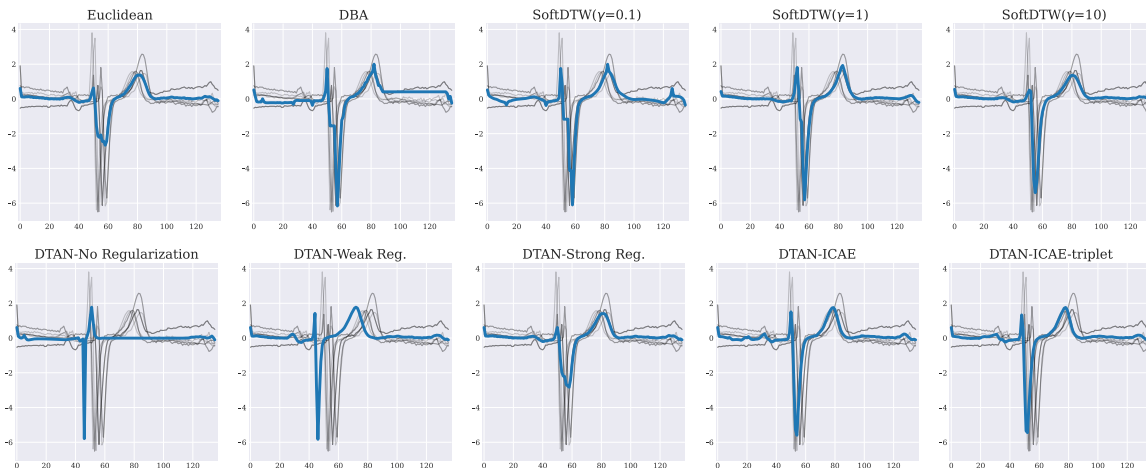
Figure 2. The effect of the regularization HP. The figures shows 10 samples (gray) from the ECGFiveDays dataset with their estimated average (blue), and compares Euclidean averaging, DBA, SoftDTW, and several DTAN methods. DBA requires no HP but falls to poor local minima. SoftDTW’s barycenter is severely affected by the choice of its smoothing HP, \gamma : \gamma = 0.1 results in a visible ‘pinching’ effect while \gamma = 10 smoothens out peaks/valleys. DBA and SoftDTW are computed per class and do not learn how to generalize to new data, unlike DTAN which is learning-based and requires a single model for all classes. The regularization often used with DTAN has 2 HPs, (\lambda_\Sigma, \lambda_{\text{smooth}}) , where a weak regularization (\lambda_\Sigma, \lambda_{\text{smooth}} : .5, .01) is insufficient and a strong regularization (\lambda_\Sigma, \lambda_{\text{smooth}} : .001, .1) , is too restrictive. Our \mathcal{L}_{\text{ICAE}} and \mathcal{L}_{\text{ICAE-triplet}} are regularization-free, yet provide barycenters that represent the data well.
