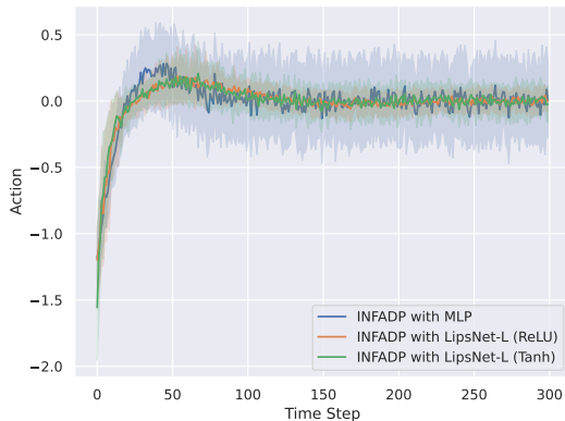
Figure 13. Action fluctuation amplitude on double integrator environment. Parentheses show the activation functions used in network f(x) .
