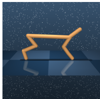
Figure 17. Cheetah(18, 6, 17) : This domain includes a planar biped. Only one task is involved in this domain, which is the run task. In this task, we need to control the planar biped to stand up and run with a forward velocity.
