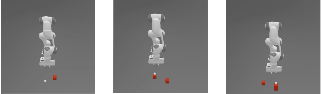
Figure 9. Examples of training time tasks. The low-level agent must follow an abstract trajectory and place a block at the designated white goal position
