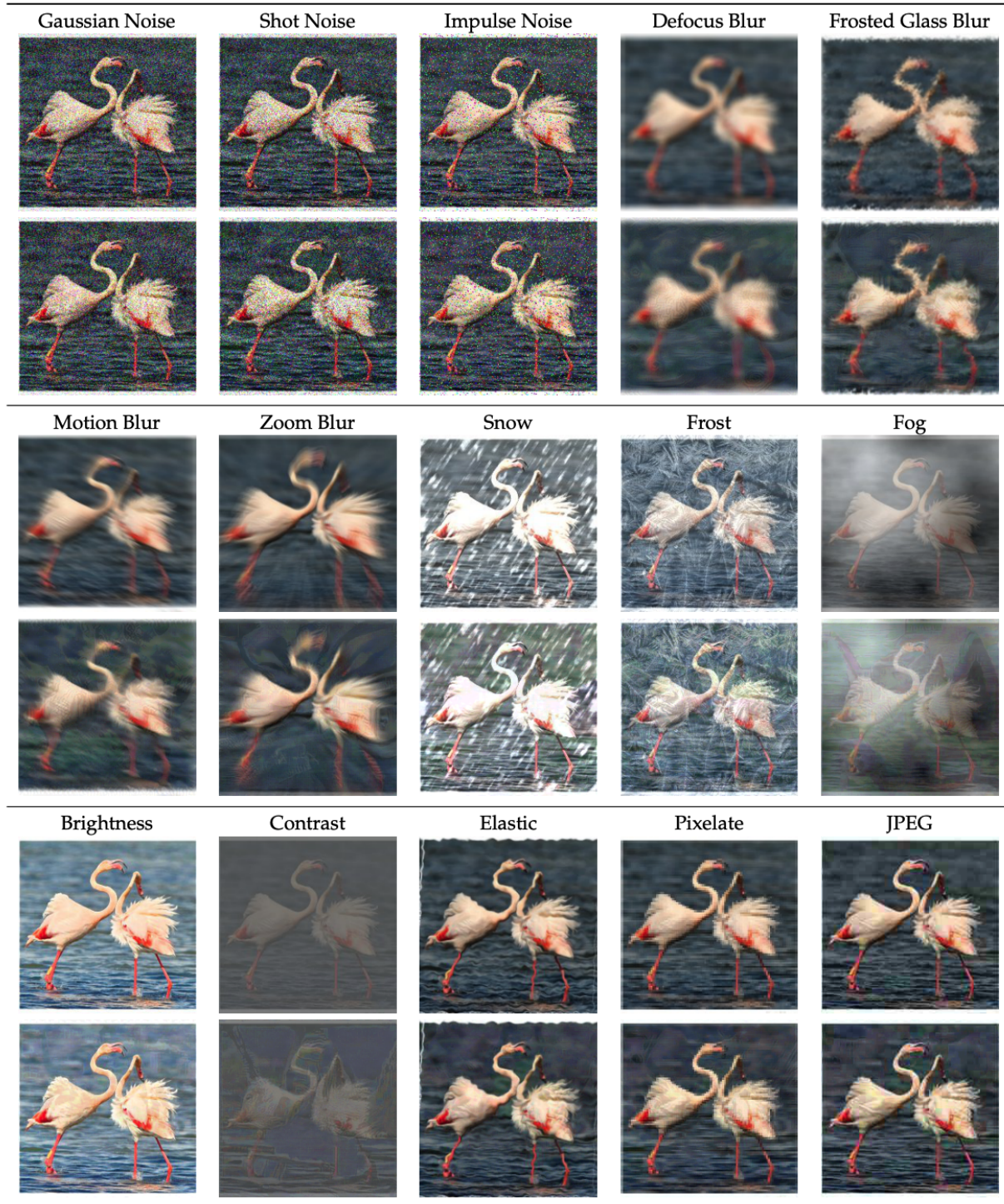
Figure 26. Demonstrations of 15 types of corrupted benign images (upper) and malicious images with \epsilon = 8/255 (lower) from the ImageNet-C benchmark. Most malicious images are visually imperceptible compared with their original ones. [Severity level: 3]
