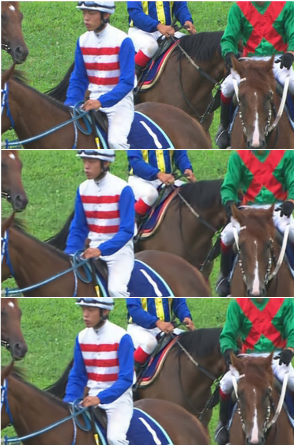
Figure 11. Qualitative results using RaceHorses of HEVC Class D. Top . Original frame. Middle . Baseline codec (DVC)'s reconstruction result with \text{bpp} = 0.448 and \text{PSNR} = 30.48\text{dB} . Bottom . Proposed method's reconstruction result with \text{bpp} = 0.379 and \text{PSNR} = 31.92\text{dB} .
