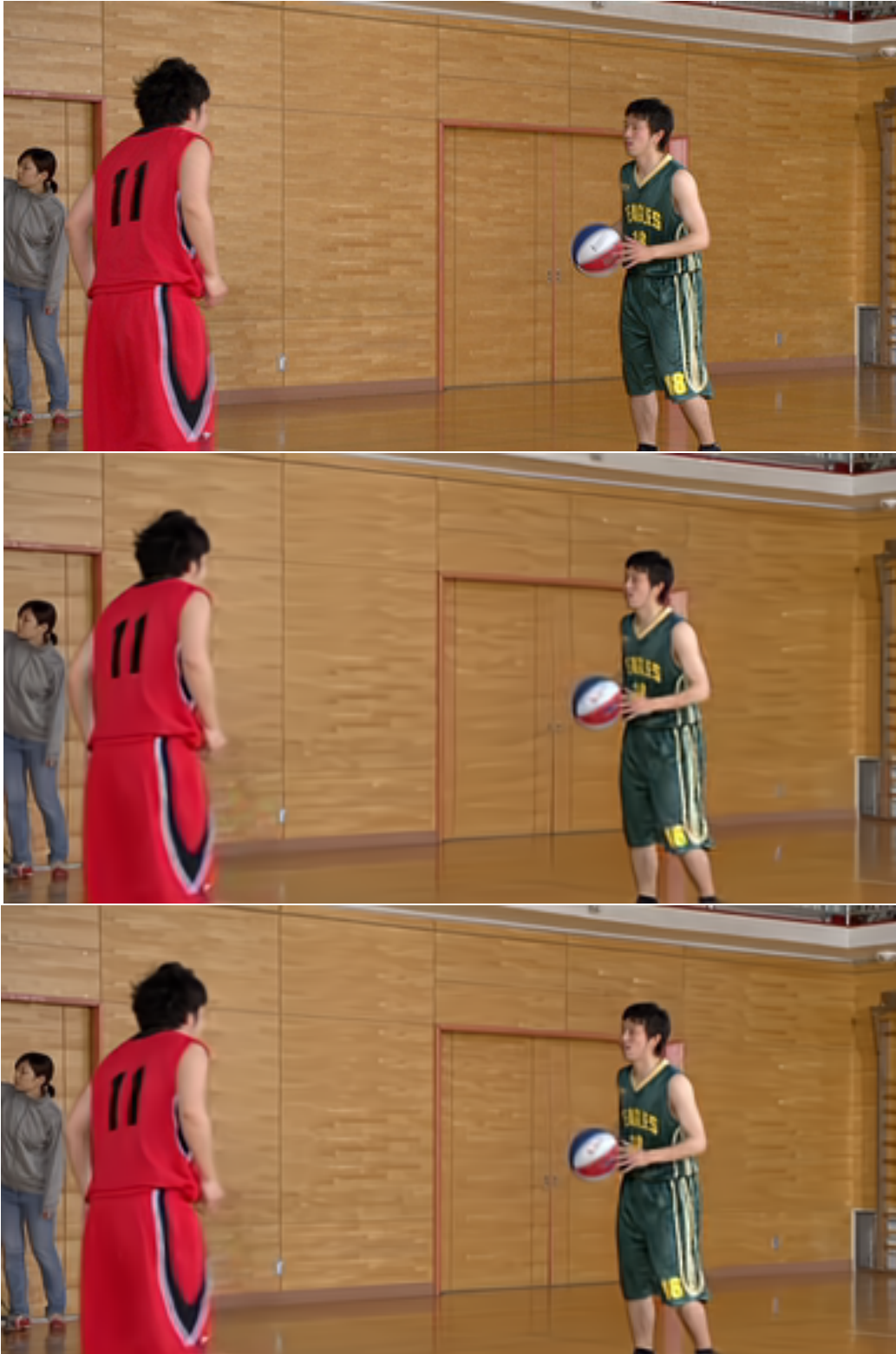
Figure 8. Qualitative results using BasketballPass of HEVC Class D. Top . Original frame. Middle . Baseline codec (DVC)'s reconstruction result with \text{bpp} = 0.148 and \text{PSNR} = 33.06\text{dB} . Bottom . Proposed method's reconstruction result with \text{bpp} = 0.103 and \text{PSNR} = 34.91\text{dB} .
