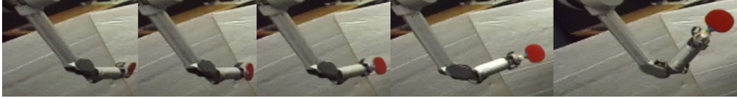
Figure 1: Frames of a 90% Topspin + 10% Lob mixture (full video available in the supplementary video). It is seen in the motion that the paddle starts in a tilted motion (standard for a topspin strike) and curves upward to return a ball with high curvature (typically of a lob strike). The location of the paddle also moves from low to high, which fits the characteristics of a lob strike.
