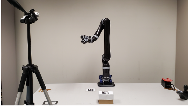
Figure 14: Experimental setup for the real robot experiments with a Kinova Jaco Gen 2 arm, [37]. An overhead Intel RealSense camera tracks an Aruco marker on the table to calibrate its 3D position w.r.t the world. It also tracks an Aruco marker on the block to extract its position.
