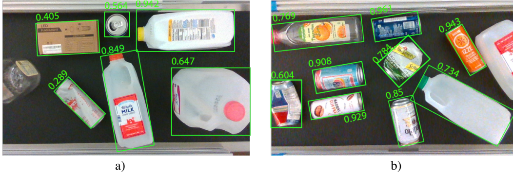
Figure 9: Sample Qualitative Results from our Robot System: Similarity scores of objects on the conveyor belt obtained from our method, when the human trained the system with 30 objects of type a) half-gallon milk jugs b) un-crushed cans
