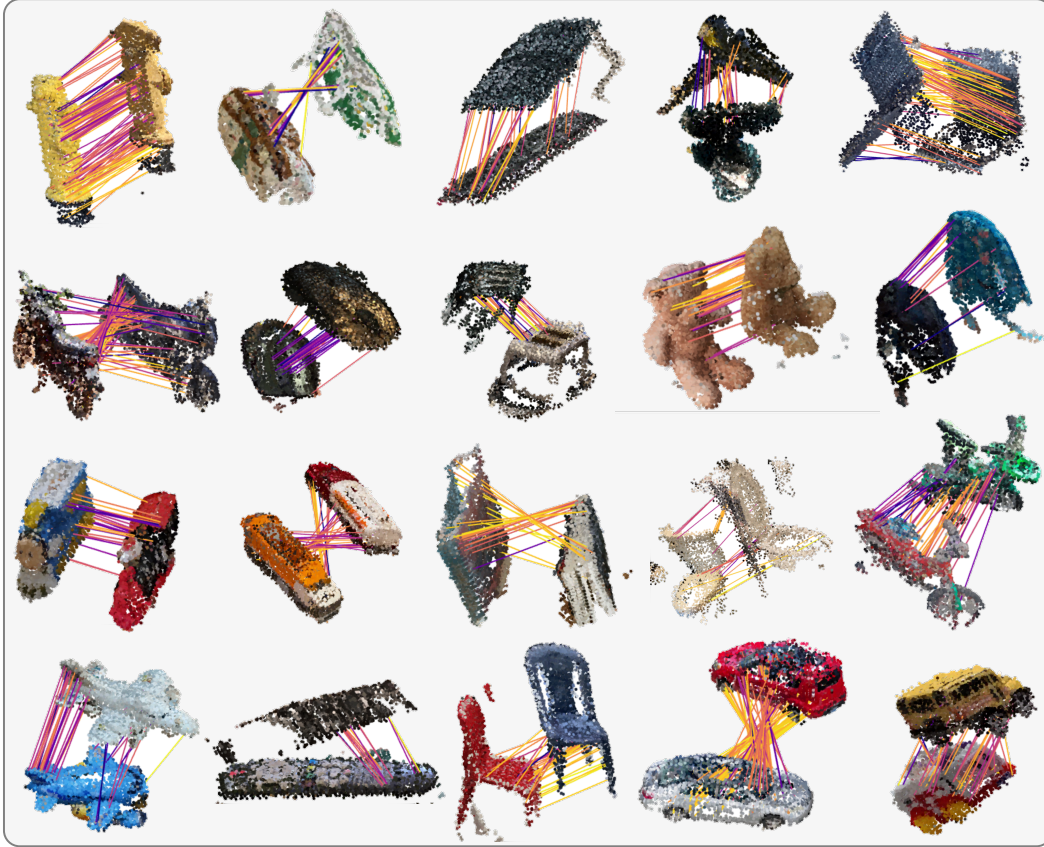
Figure A.3: An example reference-target object pair from each of 20 CO3D categories used for pose estimation. Point clouds are created from the images and depth maps as described in Section 7.4.2. Point clouds are rendered with respect to the camera viewpoint of the first frame in their respective sequences, with an added fix offset to avoid overlap. Lines between the objects show the inlier set of correspondences following the RANSAC rigid body solution (Section 3.4.2). As in Fig. 2, line colour shows correspondence similarity (■ =higher, ■ =lower). Categories, from left to right, top to bottom: hydrant, handbag, keyboard, hairdryer, laptop, motorbike, mouse, toaster, teddybear, backpack, toy train, toy bust, book, toilet, bicycle, toy plane, remote, chair, car, toy truck .
