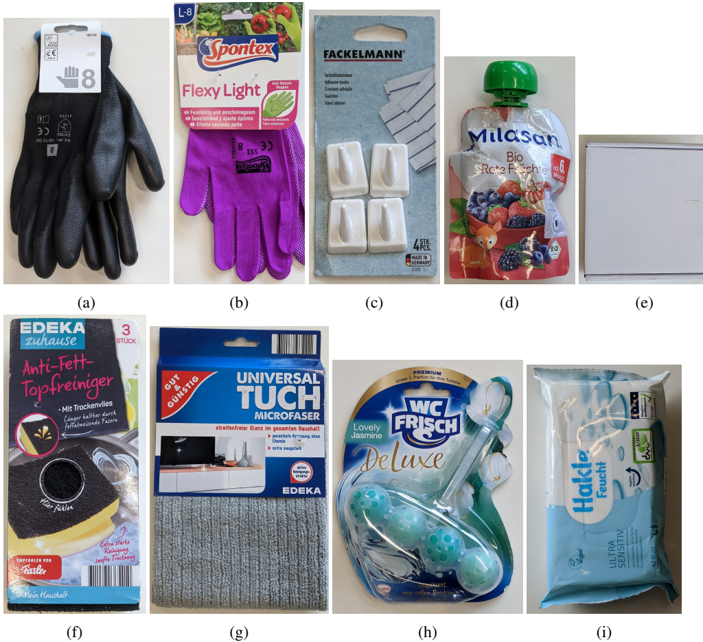
Figure 14: We used nine different objects in the grasping experiment. Some of these objects are prone to fail when planning the grasp based on 3D geometry. In other cases a suction grasp may damage parts of the objects. Therefore, using grasp preferences both improves grasp success and avoids damaging object packaging.
