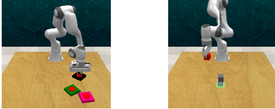
Figure 1: The tasks used in multi-variation setting. Left: push buttons task. Right: tower task.
