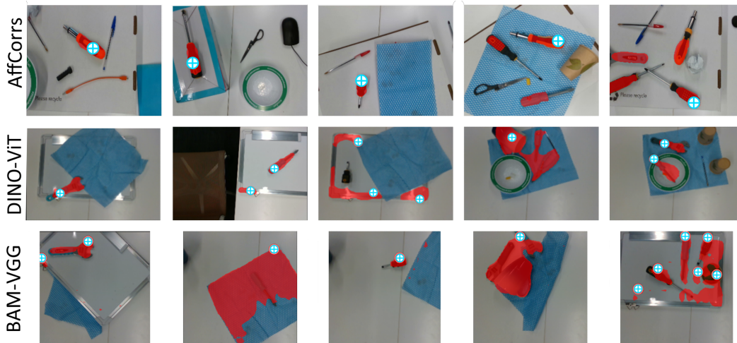
Figure 1: Comparison between the grasping points generated by the three methods, shown as blue crosshairs with corresponding areas highlighted in red. Note that the AffCorrs row only shows grasping points for the next grasp to be executed. Some baseline grasps were successful despite the correspondence being wrong (e.g., DINO-ViT, first column)
