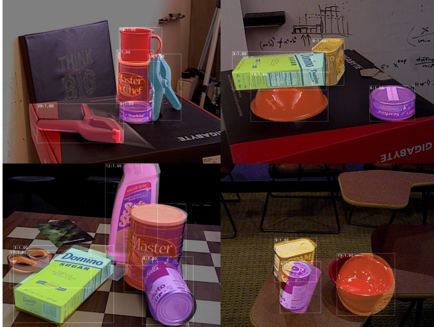
Figure 2: Qualitative results for selected frames of the YCB-V dataset. Given the relative 6D object poses predicted by PoET we project the 3D model into the image.
