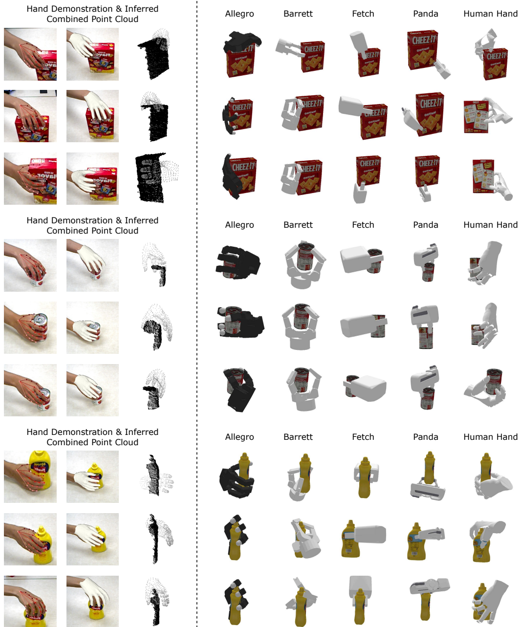
Figure 6: Closest grasps for all grippers for the human demonstrations on the cracker box (first row), tomato soup can (second row), and mustard bottle (third row).
