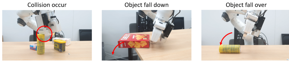
Figure 16: The representative examples of the failure cases for pushing manipulation.
