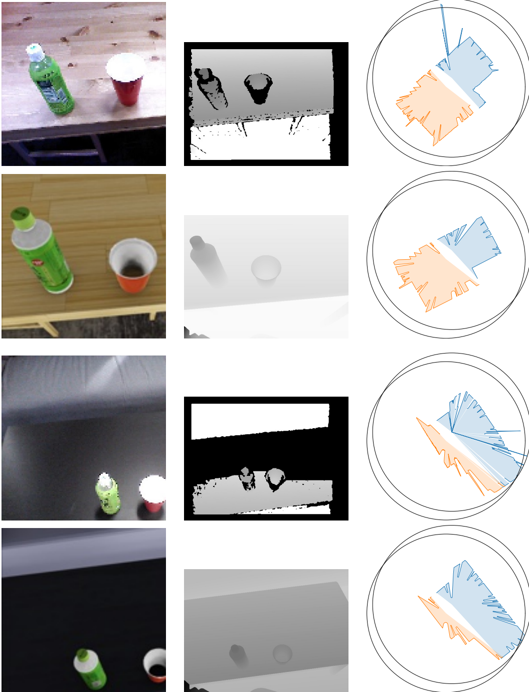
Figure A.12: Comparison between real and simulated sensor signals. RGB, Depth and LiDAR signals from the real-world sensors (first and third rows) and from the simulated sensors (second and fourth rows) at two different locations of the mockup_apr scene (location 1: first two rows, location 2: last two rows). We observed a smaller sensor sim-real gap for LiDAR than for RGB and Depth: RGB is heavily influenced by lighting conditions and camera settings while Depth has difficulty in capturing reflective surfaces.
