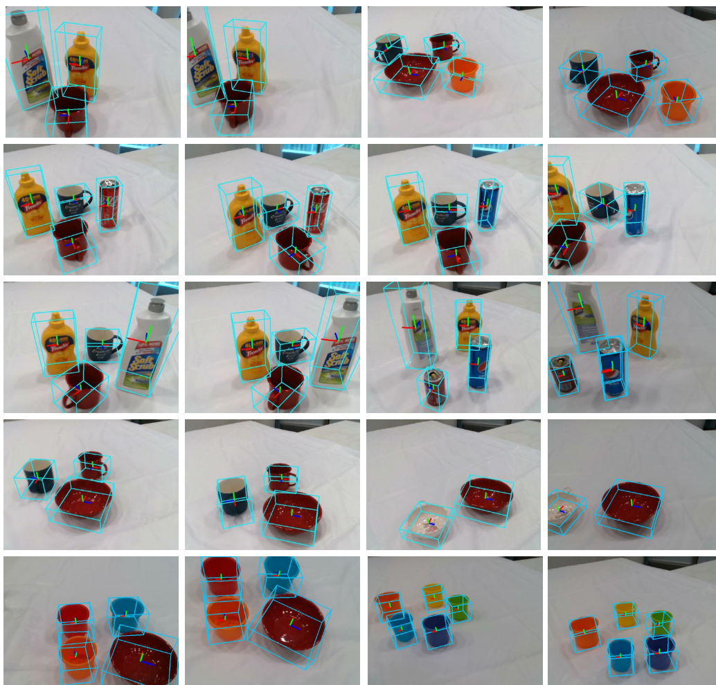
Figure G: Results of real scenes. These scenarios contain different kinds of household objects of different shapes. The objects are marked out by tight orientated bounding boxes. The red, green and blue axes represent the x, y, and z axes of the canonical coordinate, respectively.
