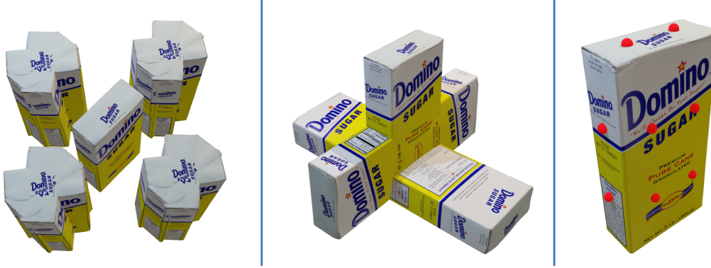
Figure 6: Subgoal generation. Left: planar subgoal poses — combination of 4 translations and 3 rotations (middle object is the original pose). Translations have been exaggerated for visual clarity. Middle: subgoals that are in neighboring stable poses (middle object is original pose). Right: Red dots are initial robot-object contact points come from a grid on the object surface.
