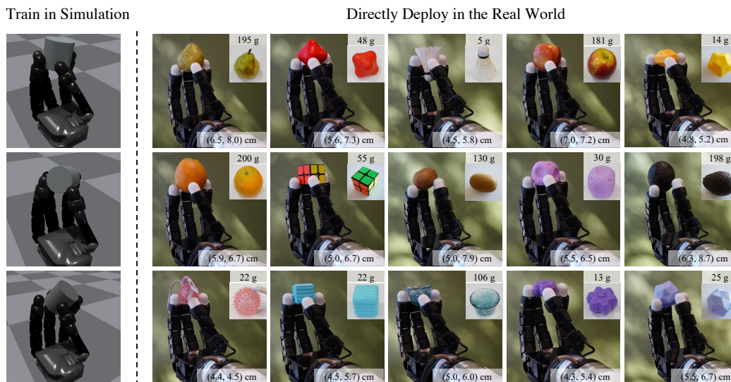
Figure 1: Left: Our controller is trained only in simulation on simple cylindrical objects of different sizes and weights. Right: Without any real world fine-tuning, the controller can be deployed to a real robot on a diverse set of objects with different shapes, sizes and weights (object mass and the shortest/longest diameter axis length along the fingertips are shown in the figure) using only proprioceptive information. Website: Emergence of natural stable finger gaits can be observed in the learned control policy.
