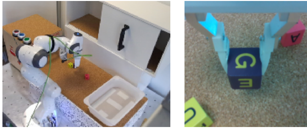
Figure 6. Visualization of the observations obtained in the real world environment. On the left we show the RGB image captured by the static camera. On the right we show the RGB image captured by the gripper camera.
