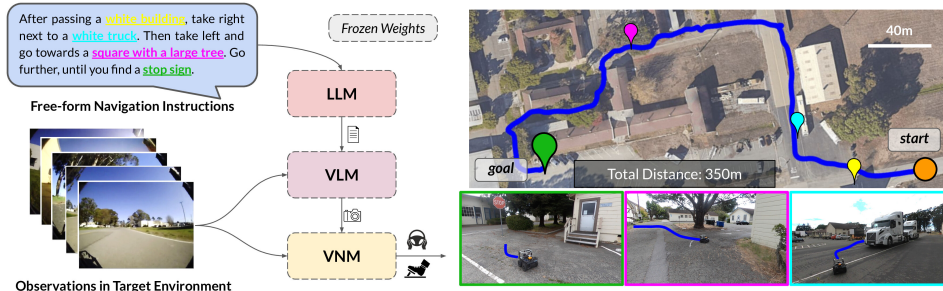
Figure 1: Embodied instruction following with LM-Nav: Our system takes as input a set of raw observations from the target environment and free-form textual instructions (left), deriving an actionable plan using three pre-trained models: a large language model (LLM) for extracting landmarks, a vision-and-language model (VLM) for grounding, and a visual navigation model (VNM) for execution. This enables LM-Nav to follow textual instructions in complex environments purely from visual observations (right) without any fine-tuning .
