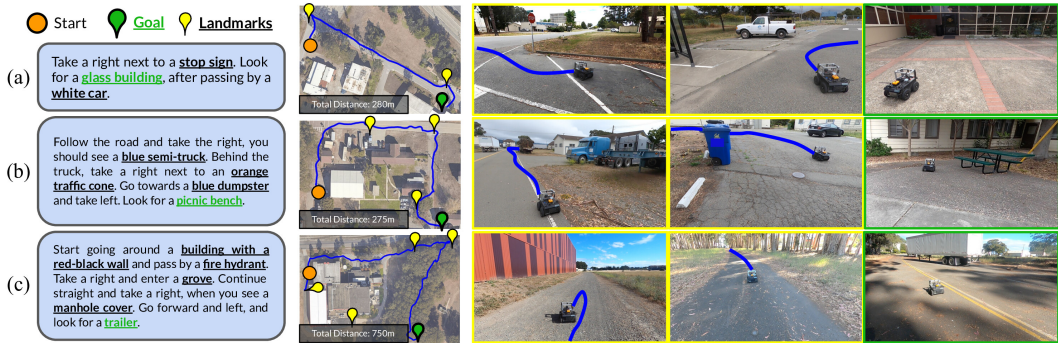
Figure 4: Qualitative examples of LM-Nav in real-world environments executing textual instructions (left). The landmarks extracted by LLM (highlighted in text) are grounded into visual observations by VLM (center; overhead image not available to the robot). The resulting walk of the graph is executed by VNM (right).
