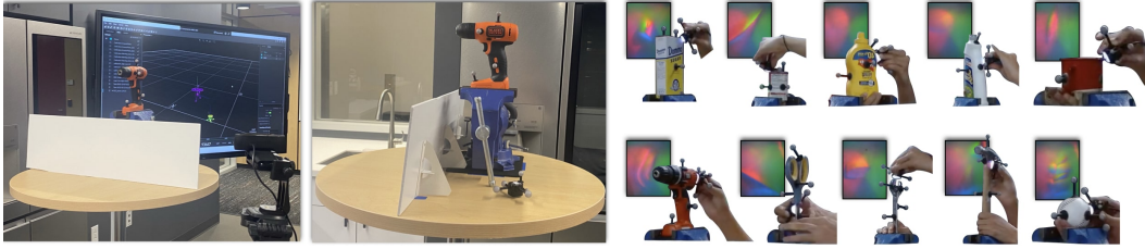
Figure 16: [left] Our data-collection setup with the YCB object, motion capture, DIGIT sensor, and recording camera. [right] The 10 YCB test objects during interactions, with representative tactile images.
