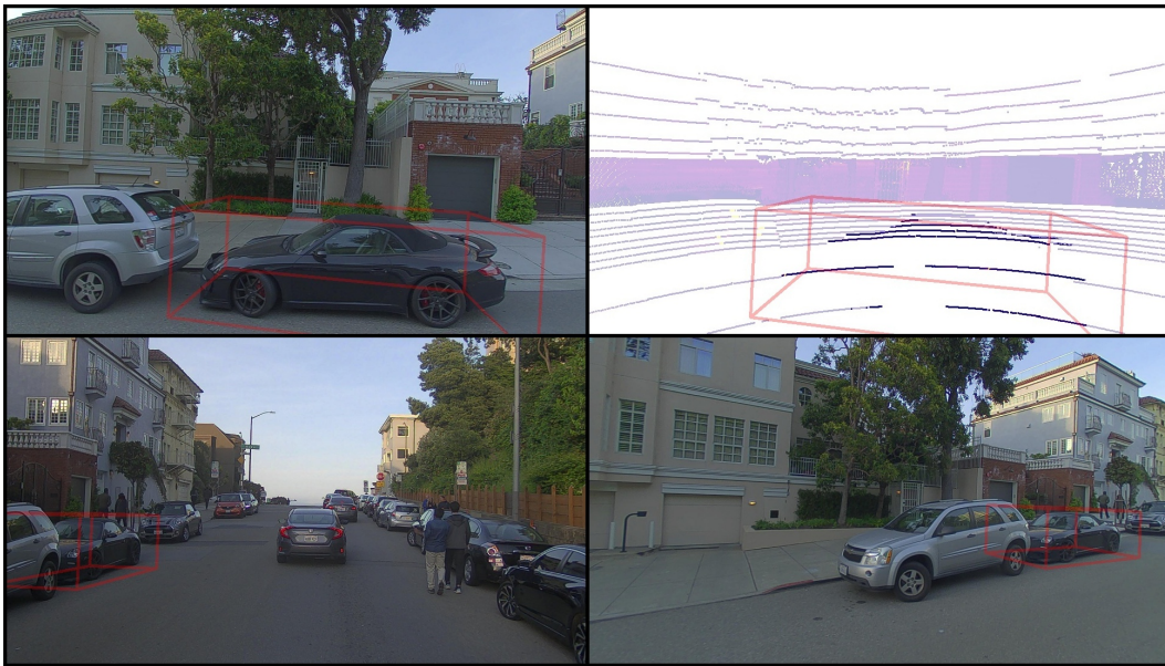
Figure A19: Illustration of vehicle 526e2f5e-e294-415c-aad6-578d27921465 (in the red bounding box) in Pandaset sequence 030. (Top) Image and LiDAR points from the left camera view used during mesh reconstruction. (Bottom) Front camera and front left camera views used during testing for the novel view synthesis task.
