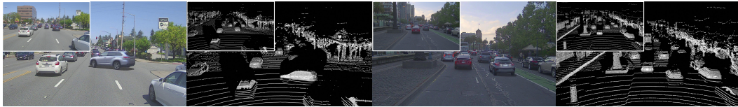
Figure 6: Multi-sensor simulation on safety-critical scenarios with animated vehicle insertion. The original camera and LiDAR observations captured in the real world are at the top-left corners.
