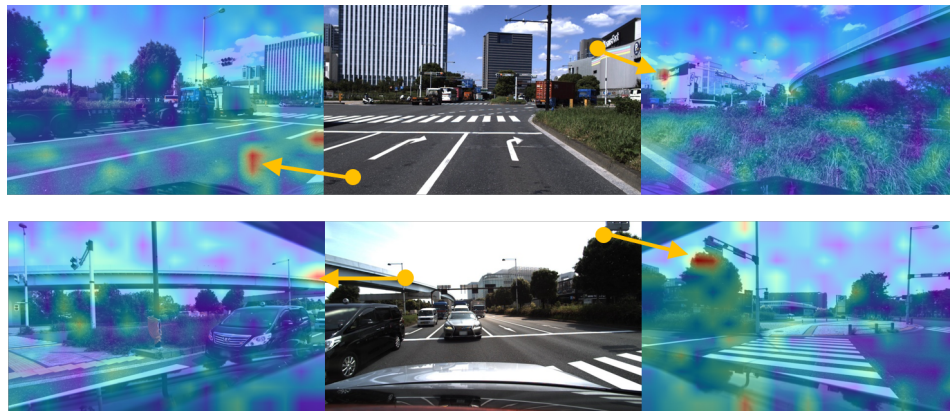
Figure 4: The visualization of cross-view attention maps. Given a set of query points, our cross-view attention maps will highlight those features at the corresponding locations in other views. The peaks of attention maps tend to appear in the overlapping areas of adjacent images, which proves that our CVT can accurately entangle the features from multiple views to achieve joint prediction. The predictions are made on the validation set at the smallest scale. Better viewed when zoomed in.
