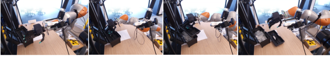
Figure 10: Learned NGF that intrinsically generates smooth motion across all 23 actuators of the robot to grasp the top tray of a toolbox and place it on the table.
