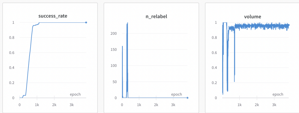
Figure 10: The progress of the performance during training. The x-axis for each figure is the number of sampled trajectories during training. From left to right: (i) Averaged success rate over a window of the nearest 20 trajectories. A trajectory succeeds if and only if the agent reaches the goal with no collision. (ii) The number of relabelled transitions along each trajectory. (iii) The ratio of admissible actions p(\phi(x, a) \geq 0), a \sim \mathcal{A} , averaged over all states \{x\} along each trajectory.
