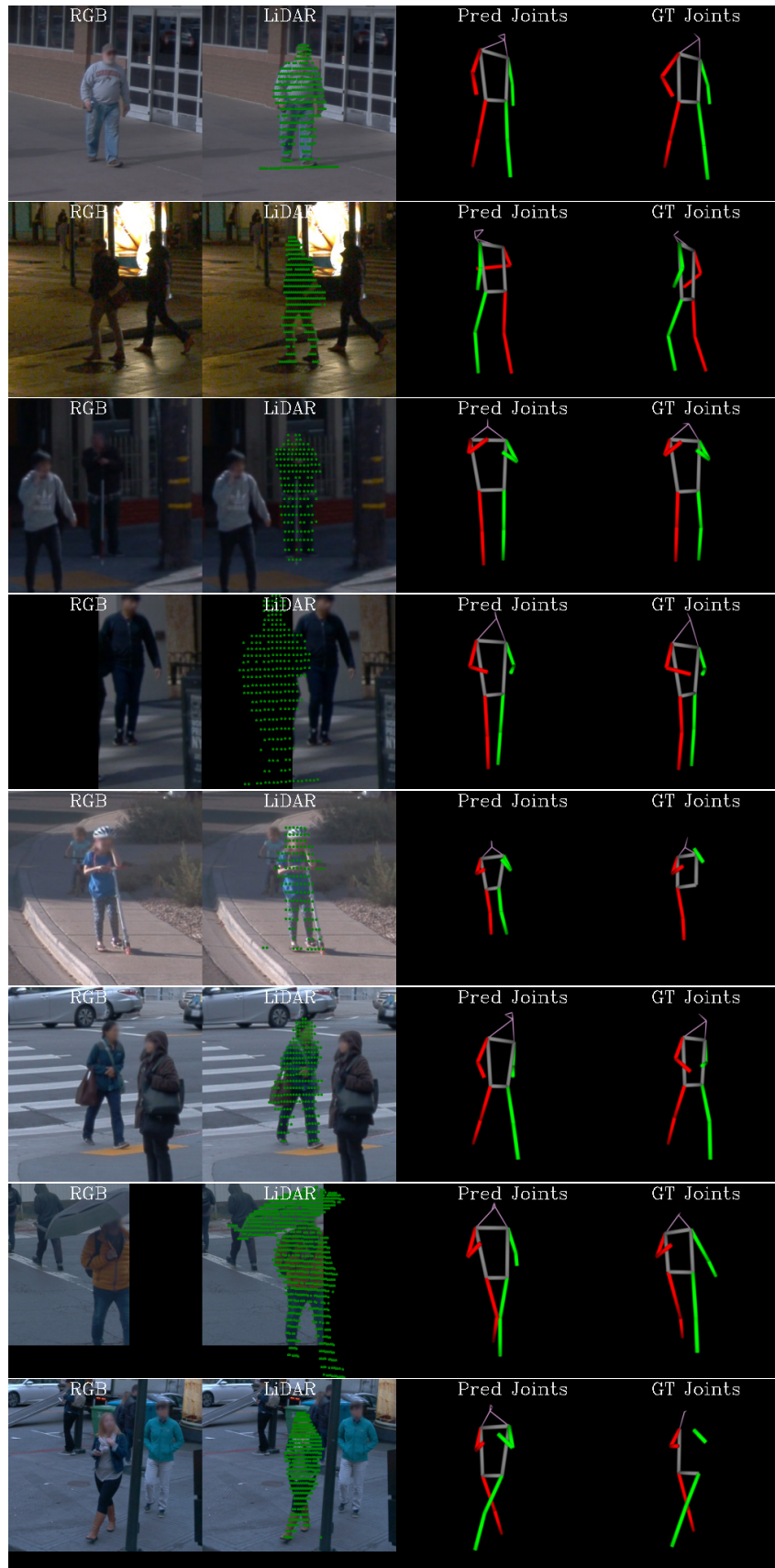
Figure 3: Qualitate results for HUM3DIL on WOD. Left to right: Input RGB, Input LiDAR, Predicted 3D joints, GT 3D joints.
