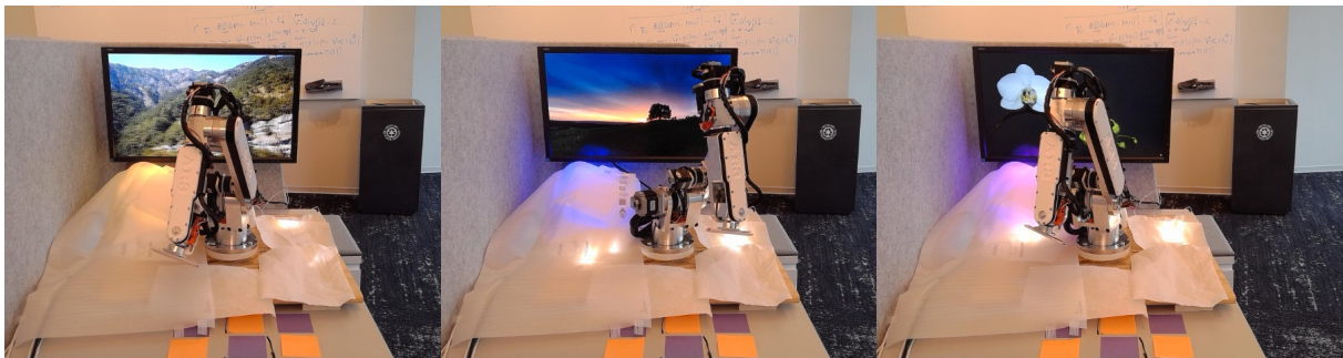
Figure 22: Experiment setup for robot data collection in presence of exogenous or irrelevant background information. Figure shows three different images, with varying background information, for the robot arm, which are part of the collected dataset.
