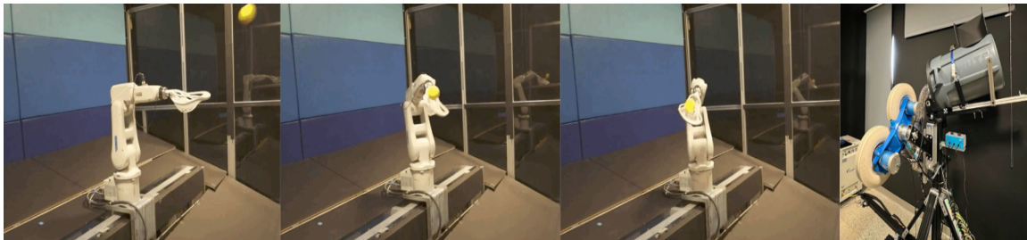
Figure 1: Mobile Manipulator with Lacrosse Head catching a ball within a second. (right) Automatic ball thrower with controllable yaw angles and speed of around 5m/s.
