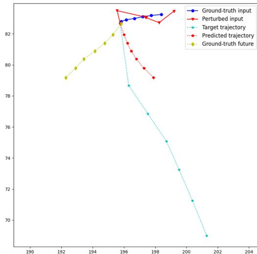
**Figure 4:** Performance of TA4TP given an aggressive target trajectory. The target trajectory requires the car to move along the cyan direction with a velocity that is significantly higher than the one associated with the input path. This difference in the velocity is illustrated by the large distance between the waypoints in the target trajectory.
