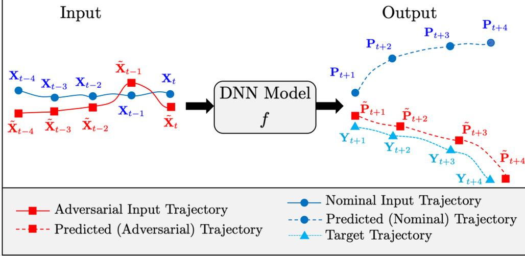
**Figure 2:** Graphical illustration of the problem formulation for  $P = F = 4$ . Our goal is to design an adversarial input trajectory (red solid line) that looks natural (i.e., close to nominal inputs - blue solid line) and fools the DNN model into predicting a trajectory (red dashed line) that is as close as possible to a desired/target trajectory (cyan dashed line).
