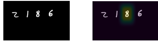
Figure 2: On the left, an example of a handwritten year. On the right, the attention map for the digit ‘8’ as a generalised normal distribution. Intuitively, we can view generalised normal distributions as differentiable bounding boxes. This allows gradients to flow from a downstream classification network to the regression component.
