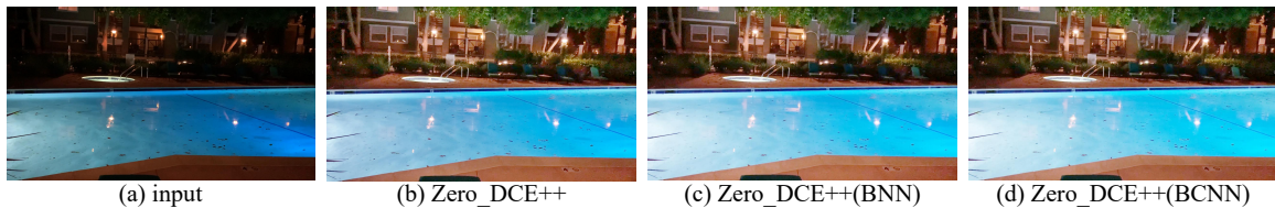
Figure 1: An example of performance from float point network and binarized networks. Zero-DCE++ Guo et al. (2020) is a low-light enhancement network. The binarized networks have similar effect with the original network with more than 85% reduction in computation and more than 83% in model size.
