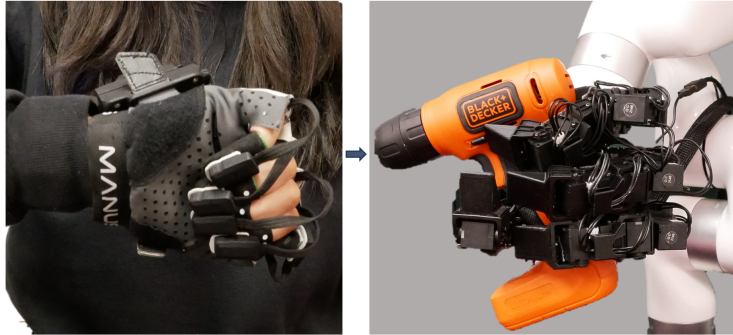
Figure 8: (left) the Manus VR glove we use to teleoperate our hand (right) the hand in the retargeted pose.
