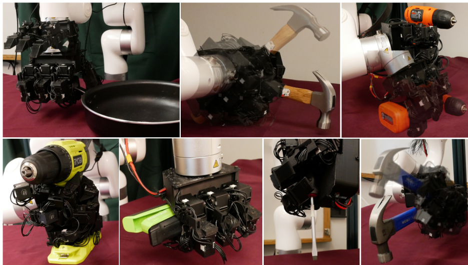
Figure 1: We use a single policy trained in simulation to pickup and grasp objects like hammers, drills, saucepan, staplers and screwdriver in different positions and orientations. An affordance model based on matching DINOv2 features is used to localize the object and move above the relevant region of the object. A blind reactive policy then picks up the object and moves it inside the palm to a firm grasp so that post-grasp motions like drilling, hammering, etc can be executed. Videos at https://dexfunc.github.io/ .
