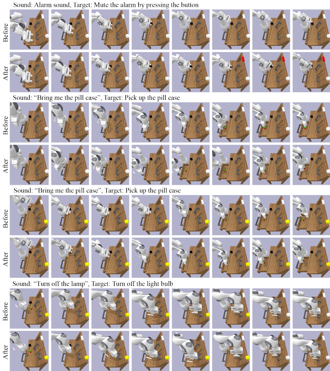
Figure 14: Visualization of the task execution in the Desk environment before and after the fine-tuning with a unseen desk and the sound commands given by new speakers. The appearance of the desk and the pill case are different from the original desk. The location of the light bulb, the button, the LED, and the drawer are different from the original desk.
