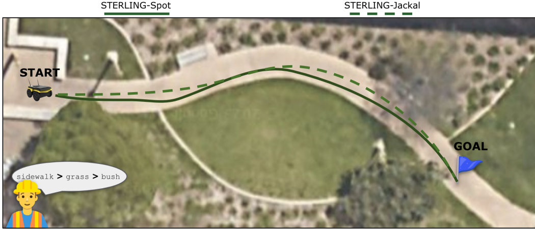
Figure 8: Experimental study of STERLING on a Clearpath Jackal—a wheeled mobile robot in Environment 6. STERLING-Spot shows the trajectory traced using STERLING trained on data collected on the Spot, deployed zero-shot on the Jackal robot, whereas STERLING-Jackal shows the trajectory traced by STERLING trained on data collected on the Jackal, deployed also on the Jackal robot. In both experiments, we see the robot reach the goal successfully while adhering to human operator’s preferences over terrains (sidewalk > grass > bush).
