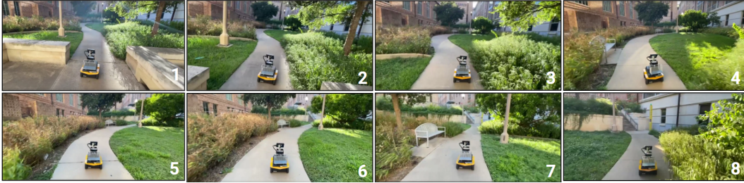
Figure 9: Clearpath Jackal, a wheeled robot navigating using STERLING features trained on unconstrained data collected on the Jackal robot (STERLING-Jackal). We see here in Env. 6 that the robot reaches the goal while adhering to operator preferences Sidewalk > Grass > Bush. This experiment demonstrates the versatility of STERLING in being applied to robots of different morphology.
