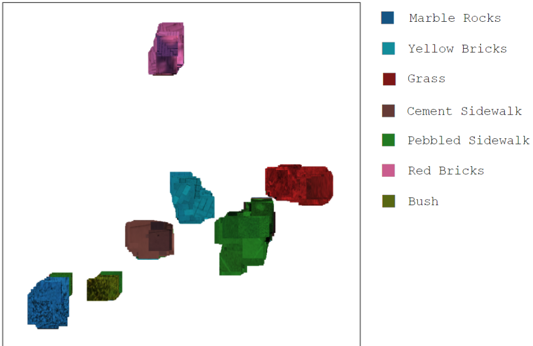
Figure 15: t-SNE visualization of terrain representations learned using STERLING. Each data point represents a terrain example, color-coded by its ground truth label. The clustering of colors shows the efficacy of STERLING in capturing meaningful and distinctive terrain features.
