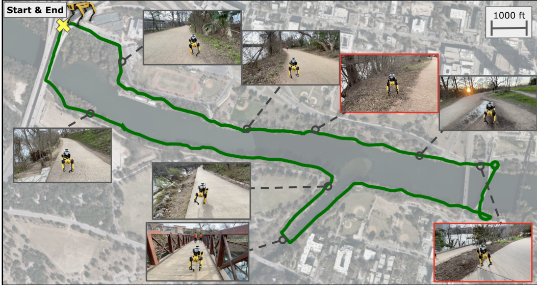
Figure 7: A large-scale qualitative evaluation of STERLING on a 3-mile outdoor trail. STERLING features successfully complete the trail with only two manual interventions (shown in red).
