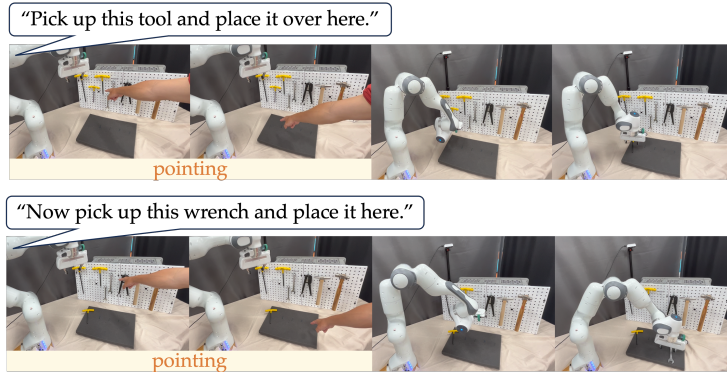
Figure 8: Fetch and place tool.
