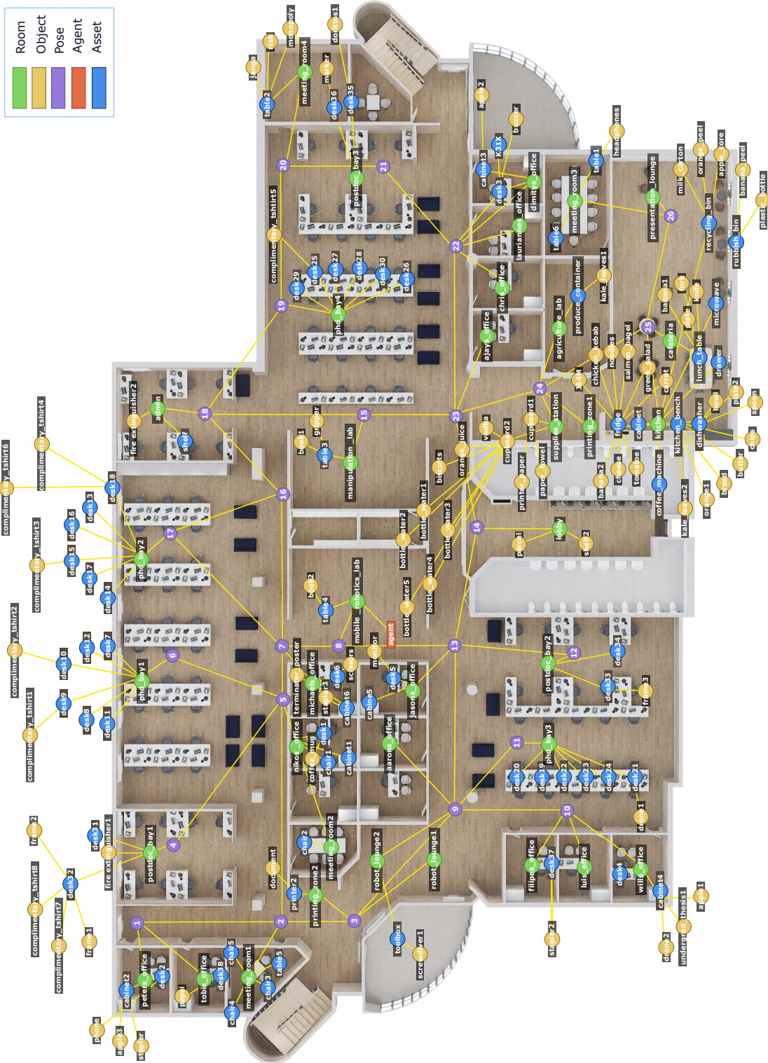
Figure 5: 3D Scene Graph - Fully Expanded Office Environment. Full 3D scene graph exposing all the rooms, assets and objects available in the scene. Note that the LLM agent never sees all this information unless it chooses to expand every possible node without contraction.
