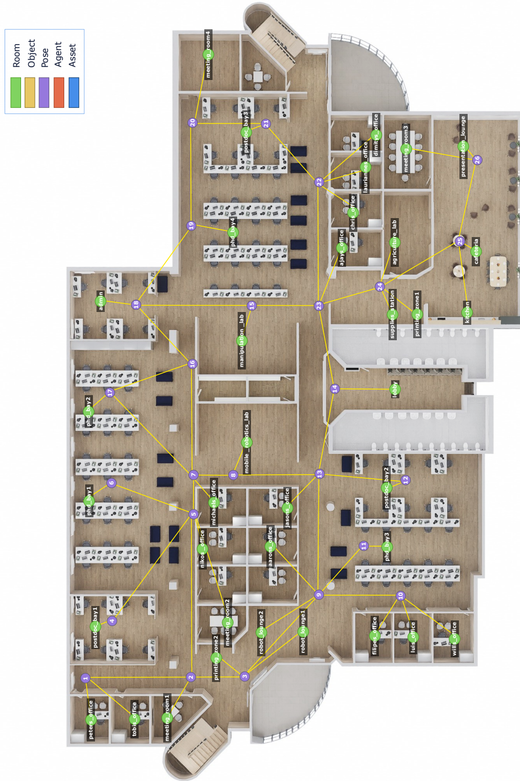
Figure 6: 3D Scene Graph - Contracted Office Environment. Contracted 3D scene graph exposing only the highest level within the hierarchy - room nodes. This results in an 82.1% reduction in the number of tokens required to represent the scene before the semantic search phase.
