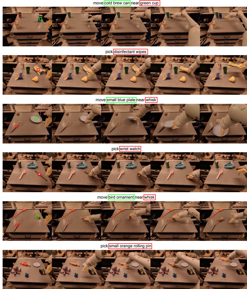
Figure 12: Example images of our policy detecting and grasping objects not seen during training time. The object detections are colored in correspondence to the text above the image, and the images are ordered left to right across time.
