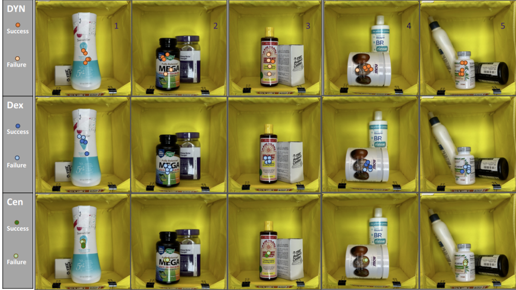
Figure 7: Real-world adversarial evaluation with five grasp points for each configuration: DYNAMO GRASP (our method), DexNet, and Centroid. The color-coded points represent the suggested grasp points success and failure from various algorithms. The successfully identified grasp points are marked by the color along the label “success” and “failure”.
