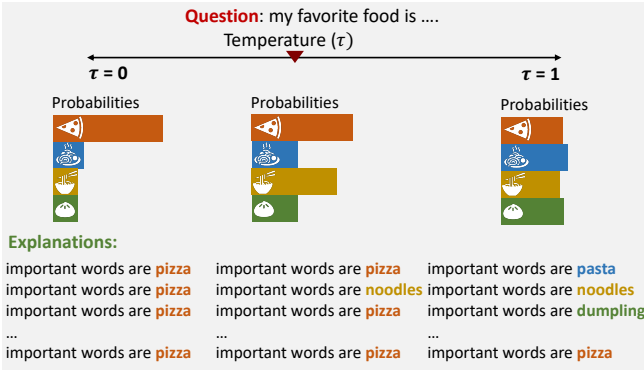
Figure 3: The impact of the temperature \tau on model stochasticity. We find that as \tau increases, the stochasticity in model responses increases. \tau=0 gives near-deterministic answers to a question, whereas \tau=1 gives a distribution of answers.
