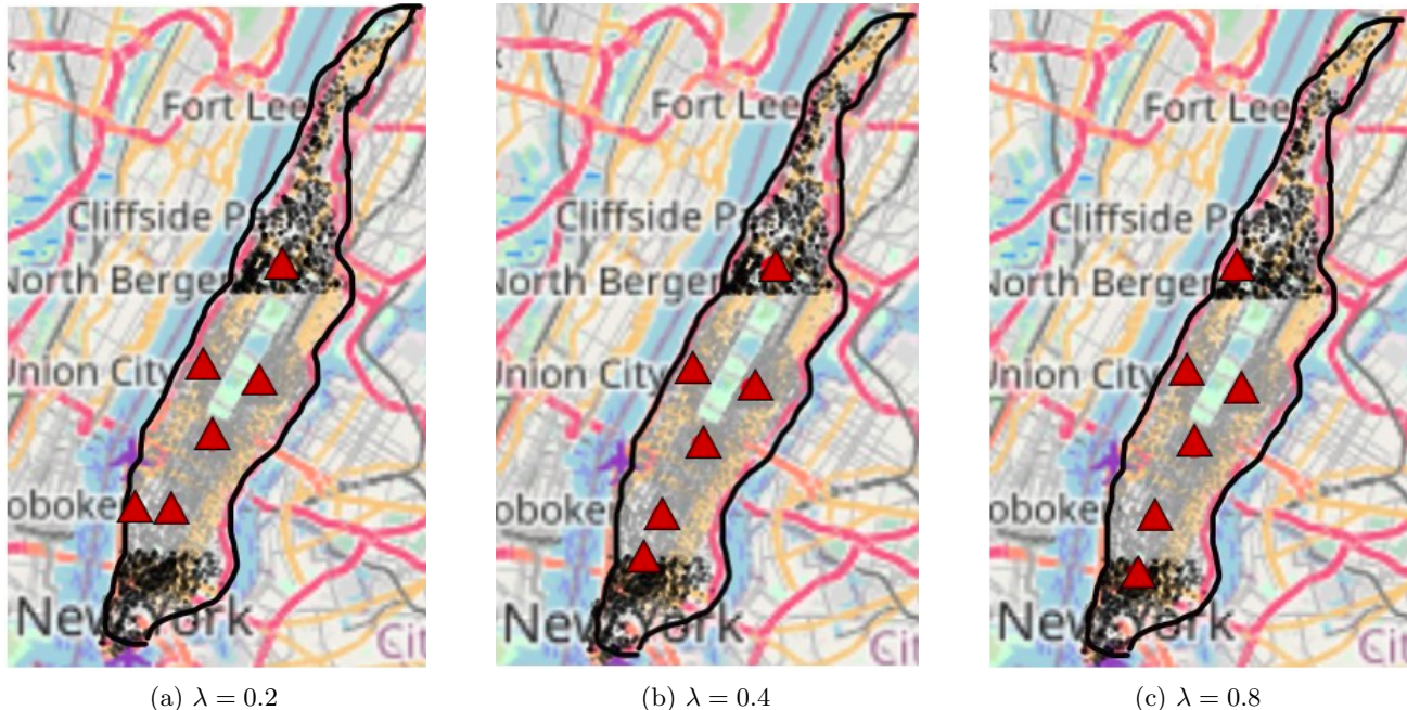
Figure 5: The results of Min-as-Oracle for 3 different values of \lambda . The red triangles represent waiting locations chosen by the algorithm, the light gray dots represent always accessible pick-up locations, and the black dots represent possibly inaccessible pick-up locations.
