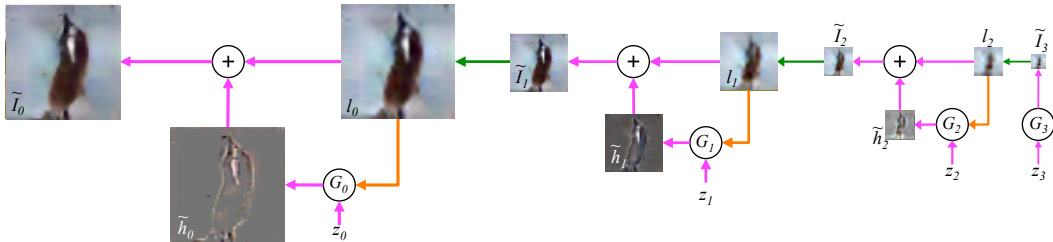
Figure 1: The sampling procedure for our LAPGAN model. We start with a noise sample z_3 (right side) and use a generative model G_3 to generate \tilde{I}_3 . This is upsampled (green arrow) and then used as the conditioning variable (orange arrow) l_2 for the generative model at the next level, G_2 . Together with another noise sample z_2 , G_2 generates a difference image \tilde{h}_2 which is added to l_2 to create \tilde{I}_2 . This process repeats across two subsequent levels to yield a final full resolution sample I_0 .
