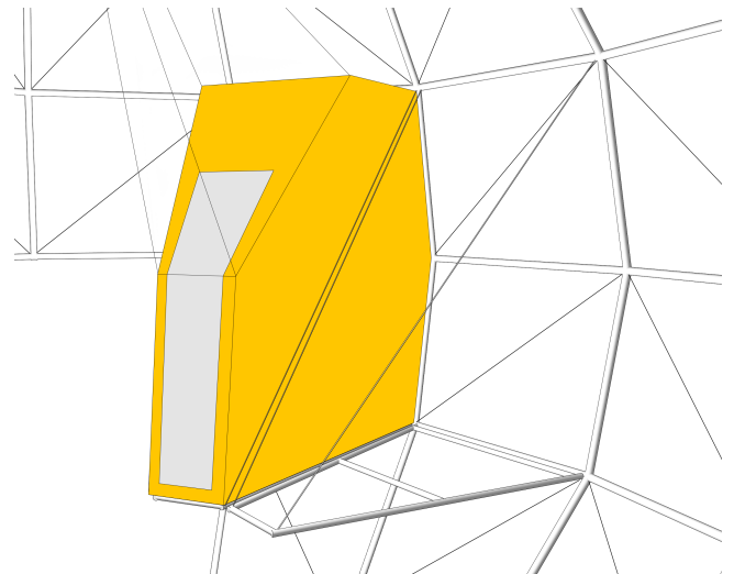
Figure 1: Mounting structure with crew quarter.
