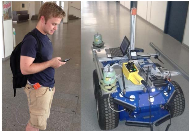
Figure 1: User with smartphone and IMU (left) and location of the sensors on the robot (right)
