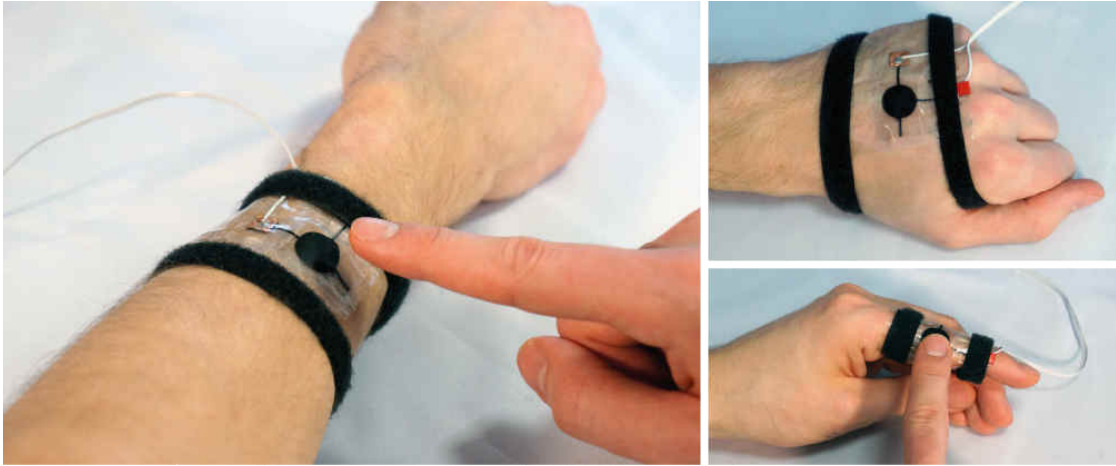
Figure 4.5: Study setup on the participants' forearm, back of the hand and finger. Two straps of Velcro allowed for fast and easy attachment.
