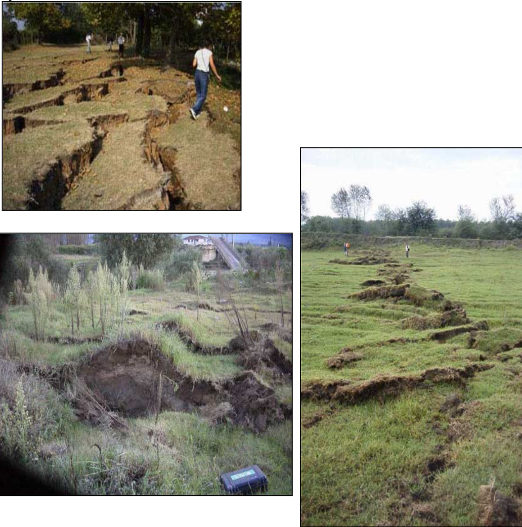
Figure I2. Photographs showing earthquake surface ruptures. Large earthquakes disrupt the ground surface in a wide variety of ways, including cracks (fissures, upper left), folds (lower left) and “mole tracks” (right) that include a variety of lateral, compressional and extensional features all mixed together. The spatial variability of ruptures both in width and along strike requires multiple excavations to truly understand the paleo-earthquake. (Photographs of ruptures from the 1999 Izmit, Turkey, magnitude 7.4 earthquake, courtesy of T. Rockwell.)
